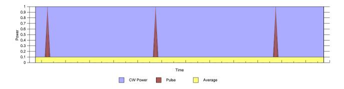
To find the radiant exposure for a single pulse, we take  $1.27 \text{ W/cm}^2$  times the 10 microseconds of exposure, and arrive at 12.7 microjoules/cm<sup>2</sup>. 100 successive pulses (a second's worth of energy) adds to a total of 1.27 millijoules/cm<sup>2</sup>. This is also equivalent to an average irradiance of 1.27 milliwatts/cm<sup>2</sup>.
