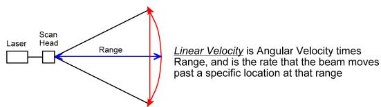
In our third example, we will use a given value of 1 centimeter for the beam diameter. If we compare the 1 cm diameter and the path length of the scan of 1000 cm, we can say that the path length is 1000 times the diameter of the beam. Moreover, since we know that this path length is traversed by the beam 100 times per second, the beam will cross its own diameter of 1 cm in (1000 cm x 100 scans per second) 1/100,000 of a second, and will be scanned 100 times in 1 second.
